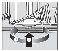
■ To remove the middle spray arm located beneath the upper basket, gently push upwards until it engages in the ratchet ①. then unscrew it ②.
